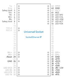
**Universal Socket Connectivity.** Multi-Tech's universal socket flexible comm-port architecture provides analog dial-up, wireless or Ethernet socket connectivity with interchangeable modules. This allows you to utilize one system design and populate it with your communication module of choice. In addition, you are assured a seamless migration to future technologies.
